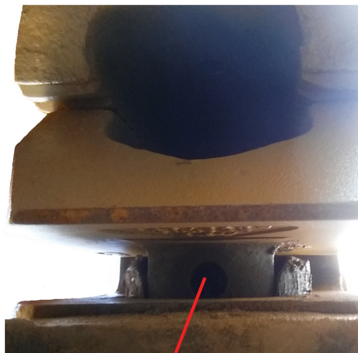
Bottom view of roll pin hole on moveable jaw
