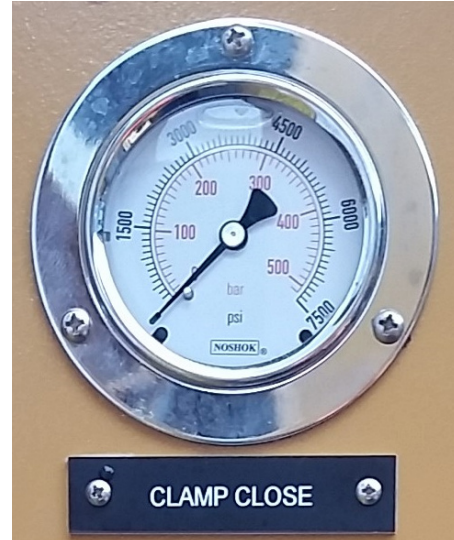
Power unit clamp CLOSE dial as seen beside the power unit control poanel. Pressure measured in psi and bar.
