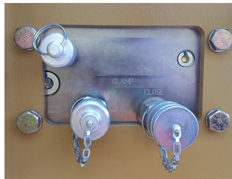
Power Unit quick disconnects, OPEN on left and CLOSE on right.
