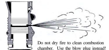
Note: Water can build up in the combustion chamber from rain or from condensation. If not removed, this water can be forced up the injector and into the fuel pump or even into the fuel tank. Water is the main source of downtime on a diesel hammer. Blow out your hammer each morning. Failure do so will result in hard starting and irregular stroke. Never dry fire a hammer as a means to remove unwanted water or oil.
