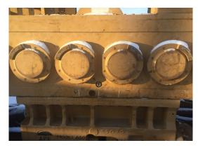
The Gear Box inside the power unit as well as the gear box in the Vibro is mandatory in cold weather to use only Neptune 150. It is Customers responsibility to ensure that appropriate oil is added when fluctuation of weather is a variable.
