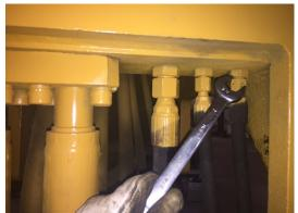
Remove the Clamp Close line at the Vibro
