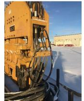
Once attached run the clamp close circuit for about 10 minutes to flush all cold hydraulic fluid from the case drain line.
