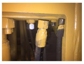
Remove the Case Drain Line at the Vibro
