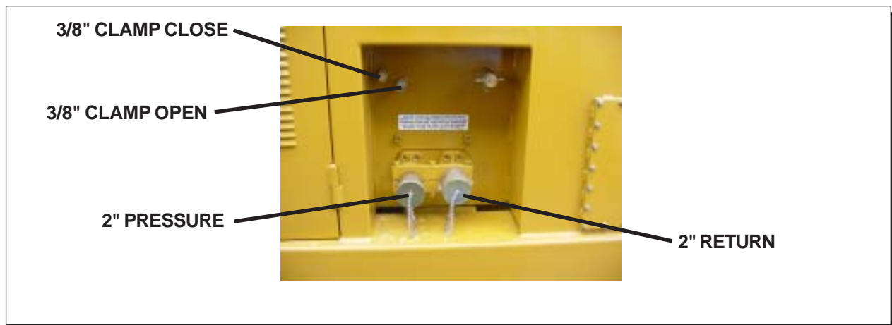
Figure 2-F. Power Unit Coupler Layout
