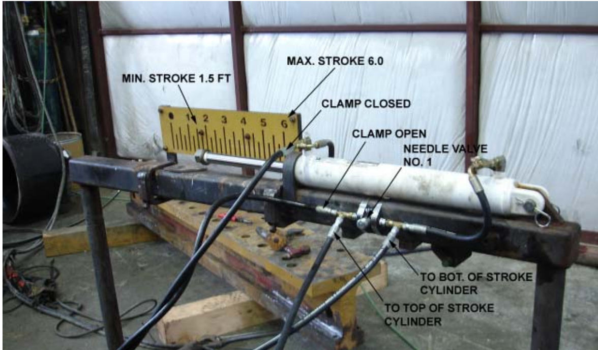
Figure 2G. Visual Stroke Indicator Cylinder
