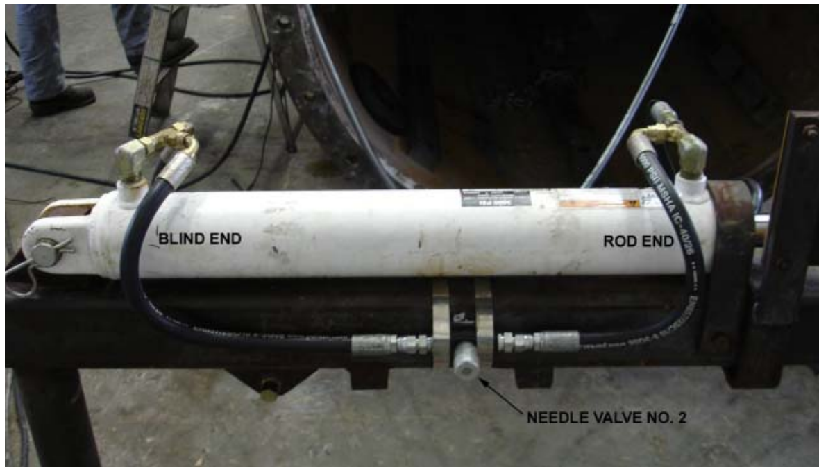
Figure 2-H. Visual Stroke Indicator Cylinder - Rear
