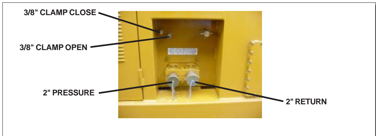
Figure 2-F. Power Unit Coupler Layout
