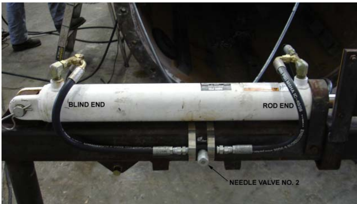
Figure 2-H. Visual Stroke Indicator Cylinder - Rear
