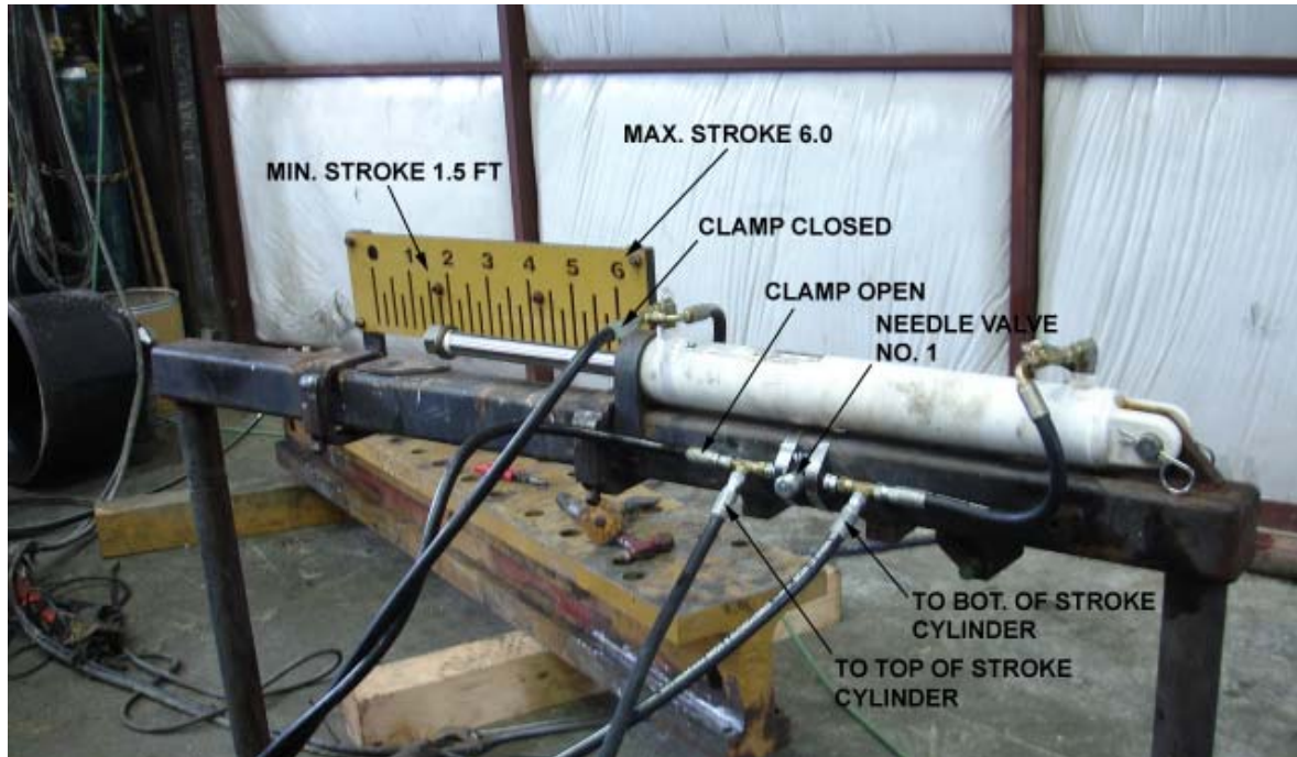
Figure 2G. Visual Stroke Indicator Cylinder
