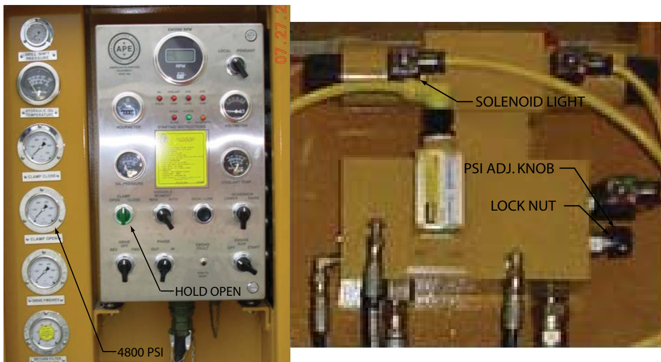
Figure 2-C. Setting Relief Valve
