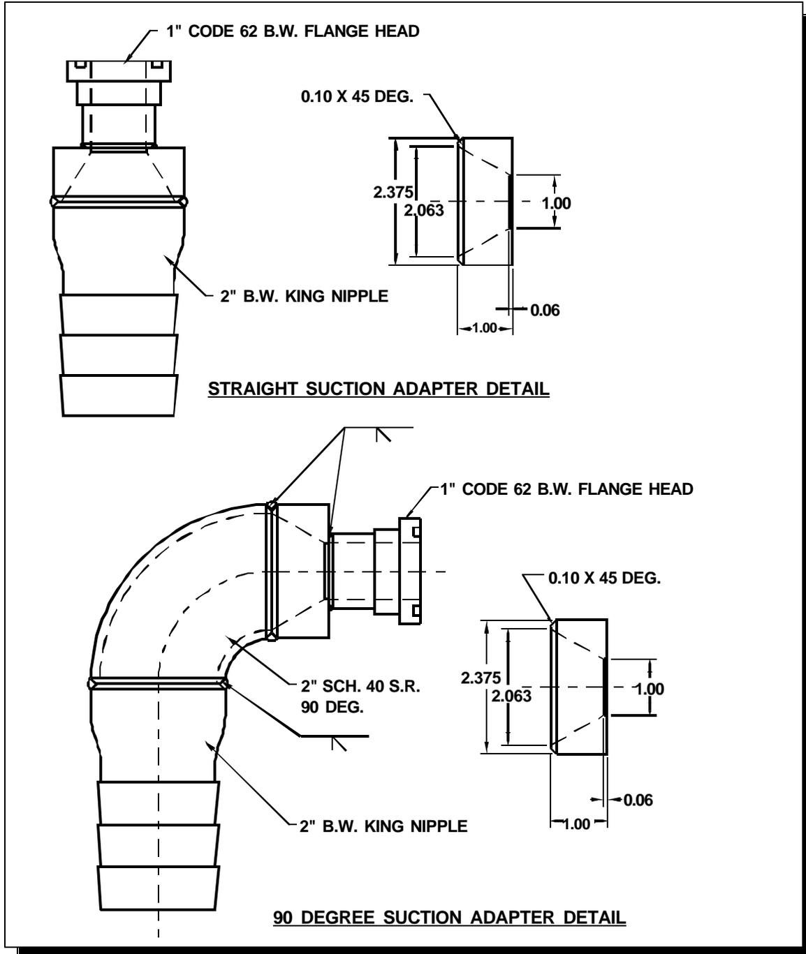
**Figure 7-F. Hydraulic Component Identification - Suction Adapter Details**
