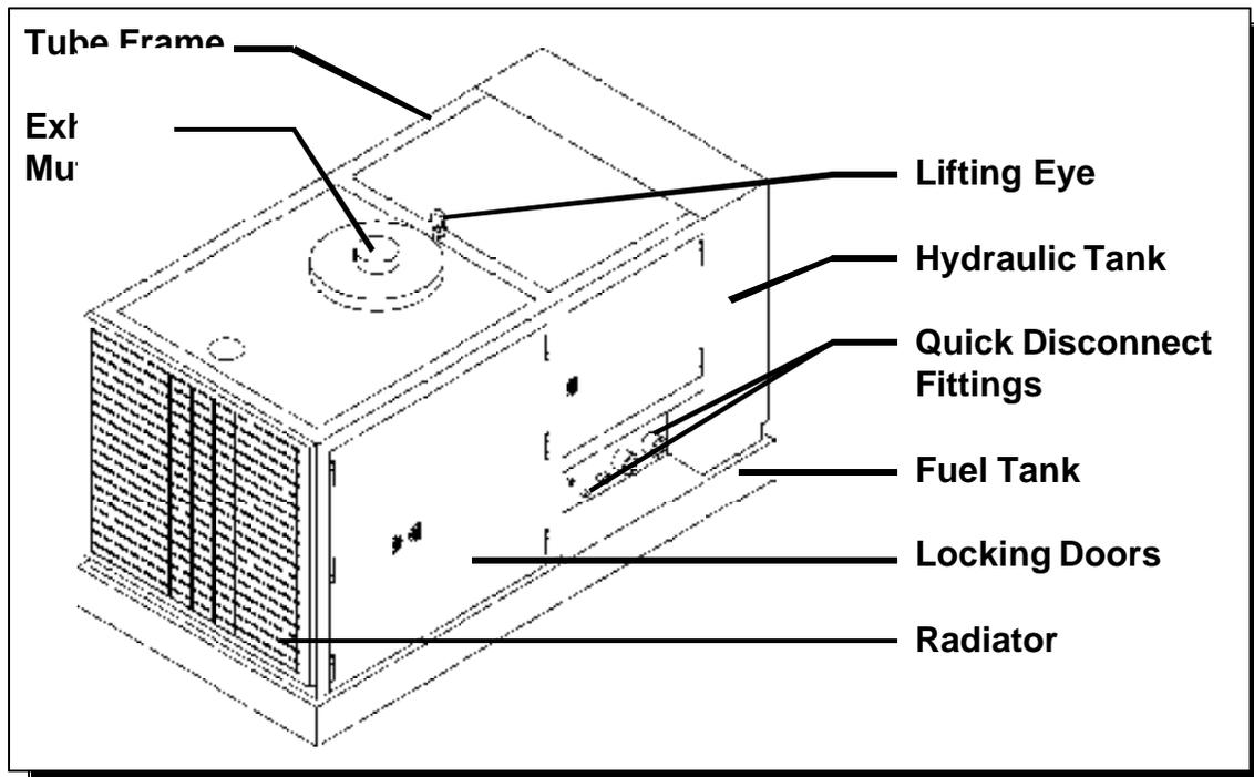
**Figure 1-H. General Description of Model 625 Power Unit**
