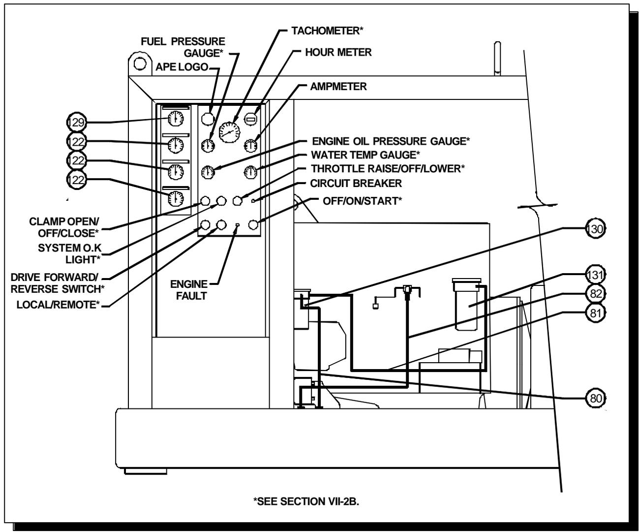
**Figure 7-D. Hydraulic Component Identification - Control Panel Detail**
