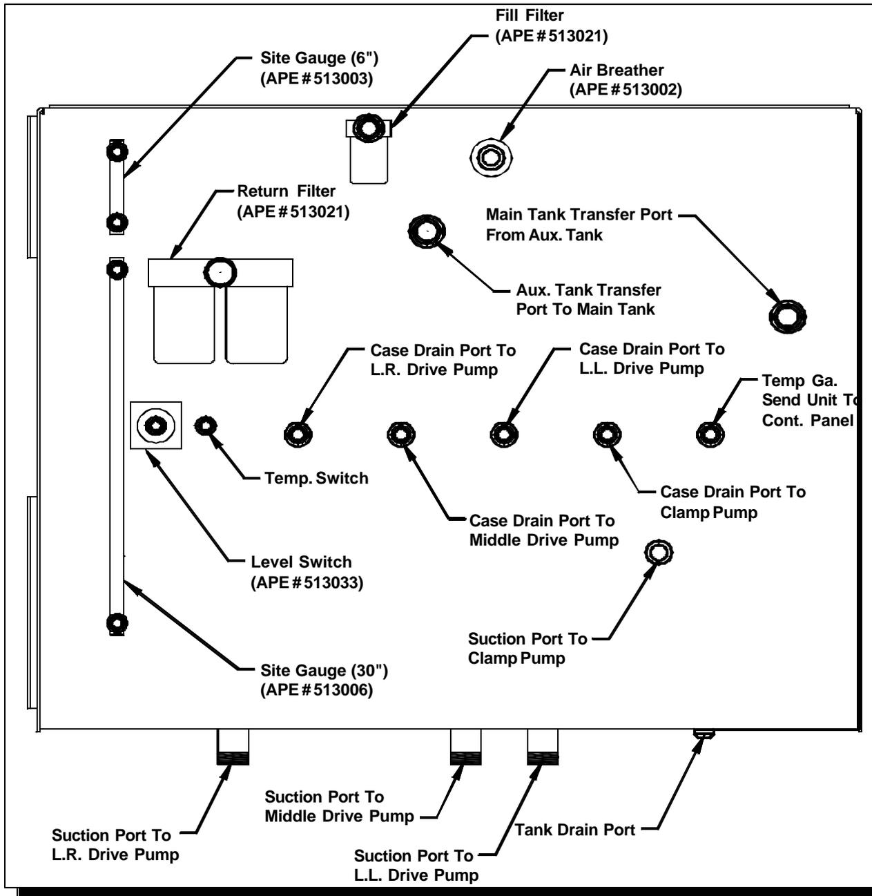
**Figure 7-E. Hydraulic Component Identification - Tank Detail**
