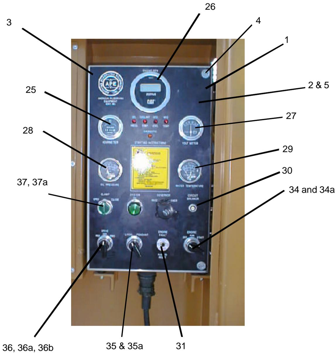
**Figure 2-G1. Control Panel Front View.**
