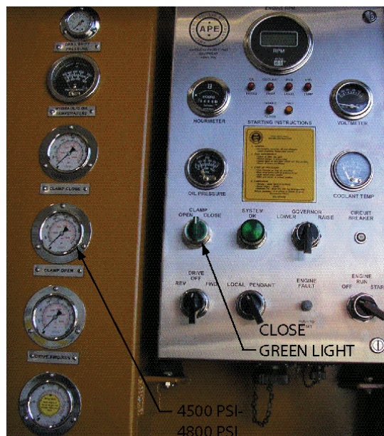
Figure 4-D. Checking Clamp Pressure Switch Setting
