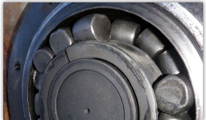
Damaged eccentric bearing in need of immediate replacement.
