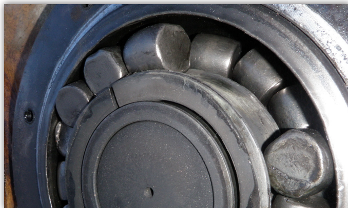
Damaged eccentric bearing in need of immediate replacement.
