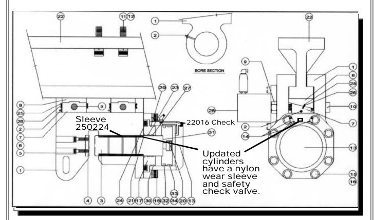
Figure 2-F. Caisson Clamp Identification.
