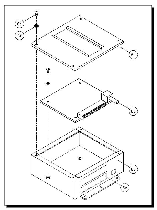
Figure 2-K2. Radio Reciever Exploded View.
