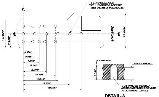
Figure 1-F. Clamp Attachment Hole Configuration
