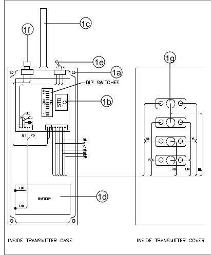
Fig 2-M1. Radio Transmitter Layout
