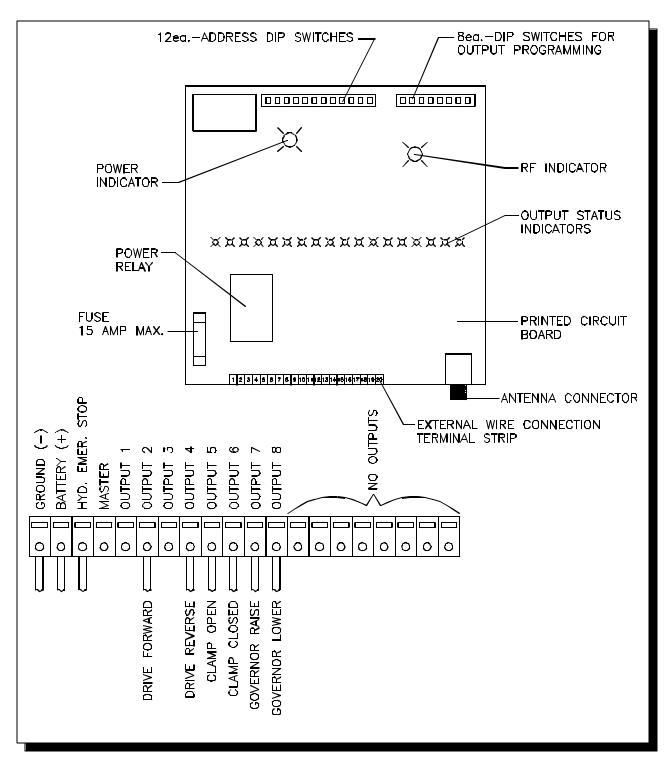
Figure 2-K3. Radio Reciever Board Layout.
