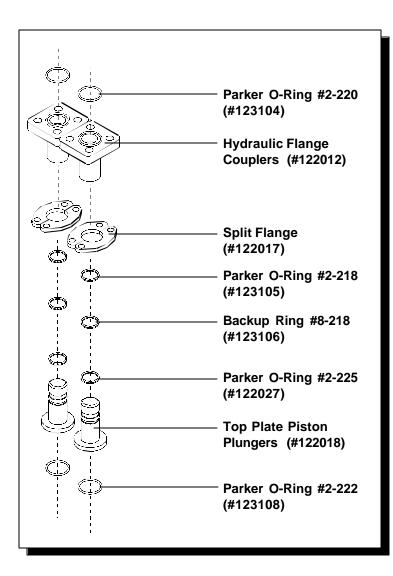
Figure 5-B. Hydraulic Motor Coupling Assembly.
