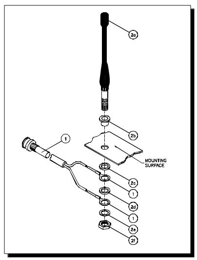
Fig 2-L. Radio Antenna Parts
