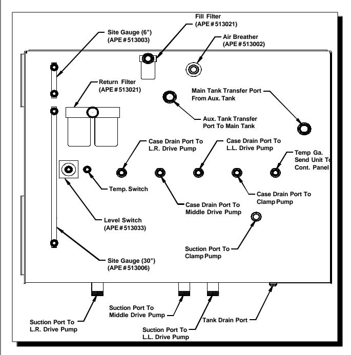
Figure 7-E. Hydraulic Component Identification - Tank Detail
