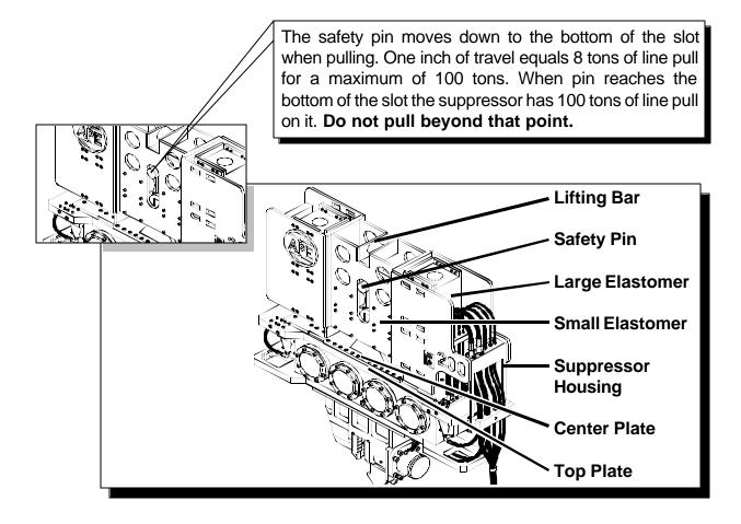
Figure 1-C. General Description of Suppressor Housing
