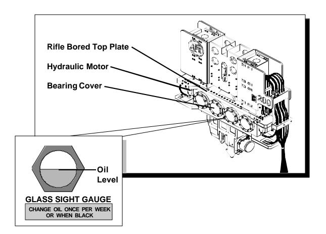
Figure 1-D. General Description of Vibrator Gearbox
