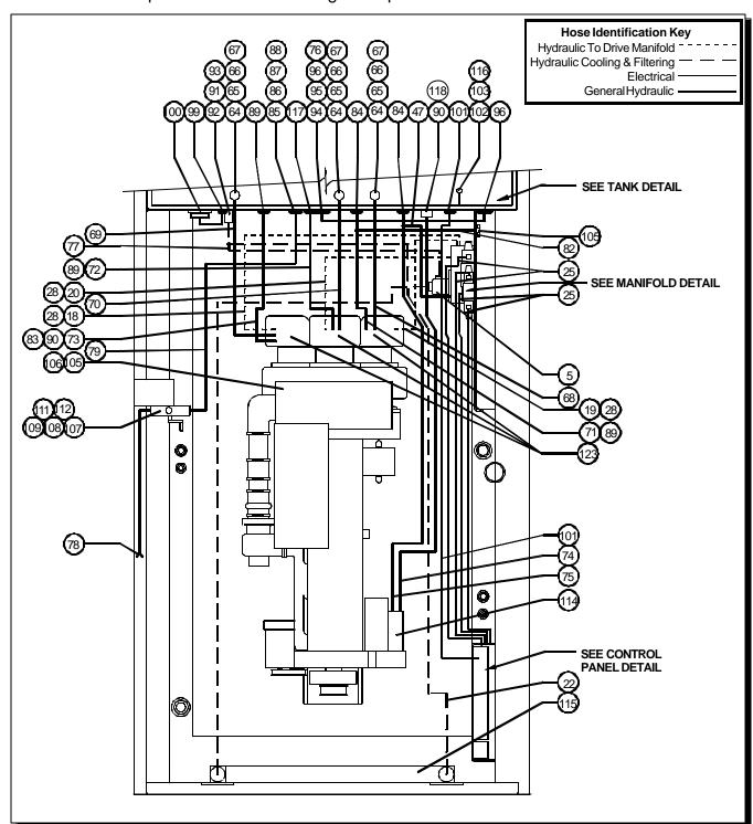
Figure 7-B. Hydraulic Component Identification - Top View
