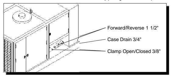
Figure 4-A. Power Unit Coupler Layout
