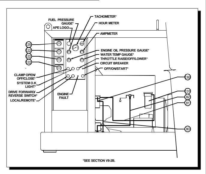
Figure 7-D. Hydraulic Component Identification - Control Panel Detail
