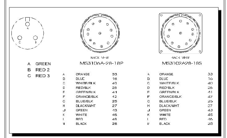
Figure 7-M. Remote Pendant Wiring Diagram
