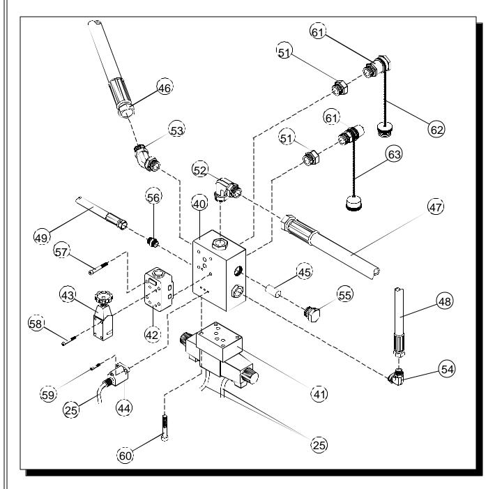
Figure 7-G. Hydraulic Component Identification - Clamp Manifold
