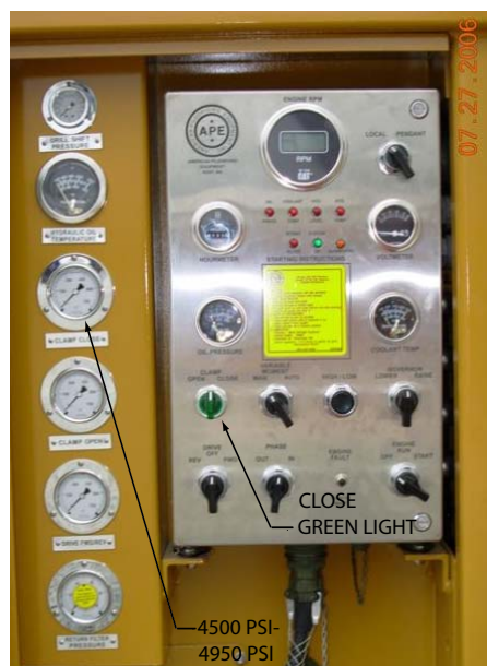
Figure 4-D. Checking Clamp Pressure Switch Setting
