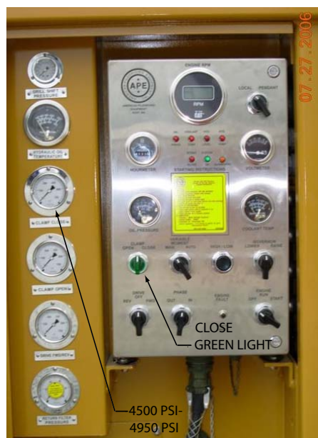
Figure 4-D. Checking Clamp Pressure Switch Setting
