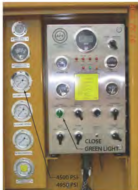
Figure 4-D. Checking Clamp Pressure Switch Setting
