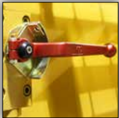
TANK TRANSFER VALVE FOR REPLENISHING HYDRAULIC FLUID
