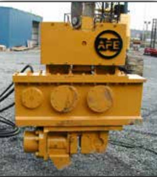
MODEL 50E WITH A STANDARD 50 CLAMP AND SINGLE/DOUBLE JAWS
