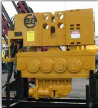
MODEL 200 VIBRO WITH A MODEL 200 SHEET CLAMP EQUIPPED WITH DOUBLE SHEET JAWS.
