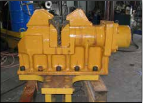
CAISSON TO SHEET ADAPTER WITH A 90 DEGREE TURN PLATE.
