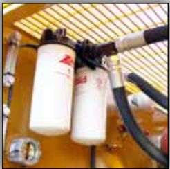
KIDNEY LOOP FILTRATION AND HYDRAULIC COOLING
