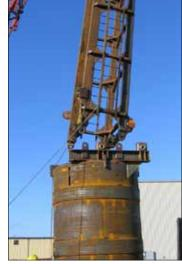
Bottom Drives for up to 12' (3.65 m) piles available including extended boots for batter/raked piles.
