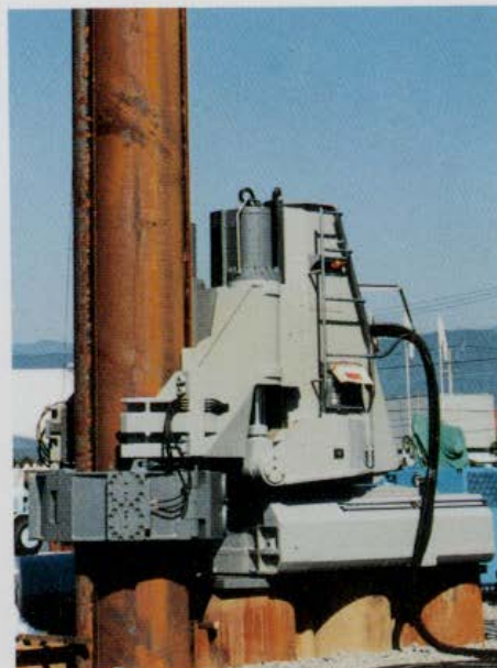
Silent Piler for Steel Tubular Piles Only
