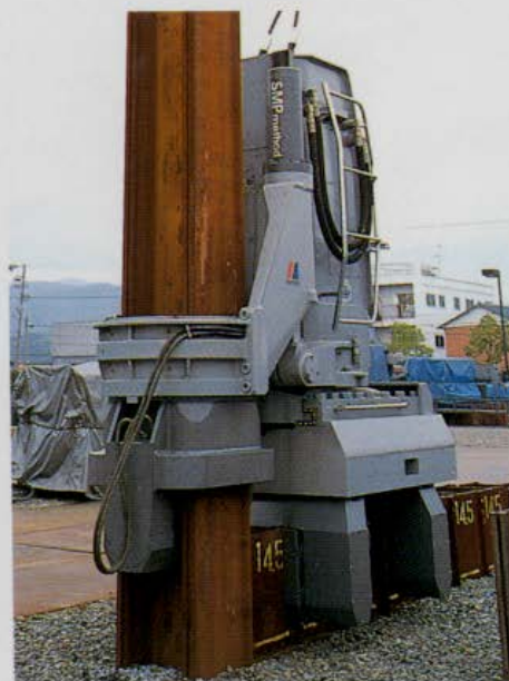
Silent Piler for H-section Steel Piles Only
