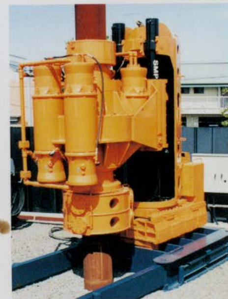
Steel Pipe Piler
