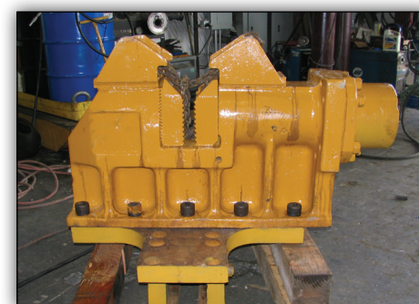
CAISSON TO SHEET ADAPTER WITH A 90 DEGREE TURN PLATE.
