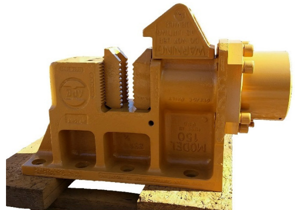
150 Sheet clamp painted for storage. Machined surface on bottom will still require protection.
